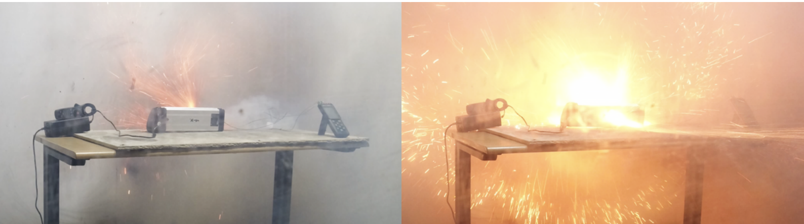
Figure 30: Photos of test sample during a thermal runaway event after being incorrectly charged.
