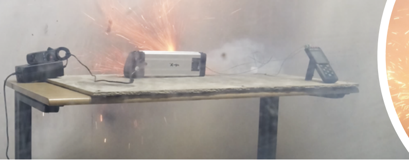
Figure 2: Photos of test sample during a thermal runaway event after being incorrectly charged.
