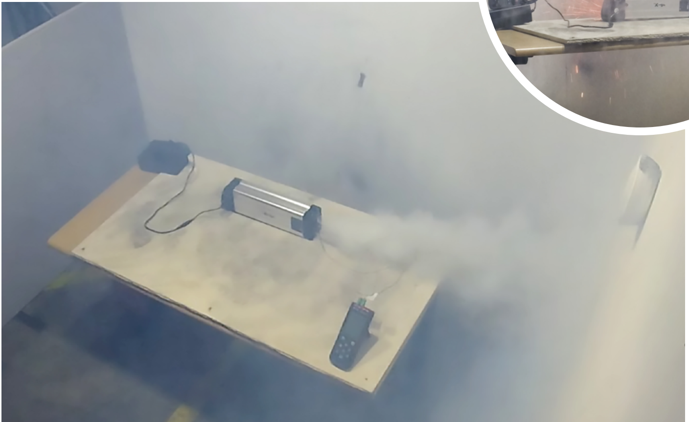
Figure 11: ©ESF Onset of thermal runaway – venting of a vapour cloud of highly flammable and toxic gases.
