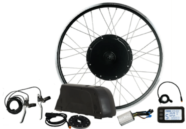
Figure 12: A typical conversion kit.
